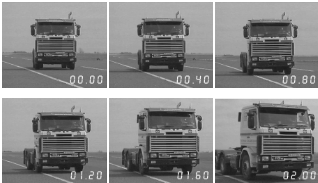
Figure 23/a Vehicle behaviour during intervention and the resulted behaviour
